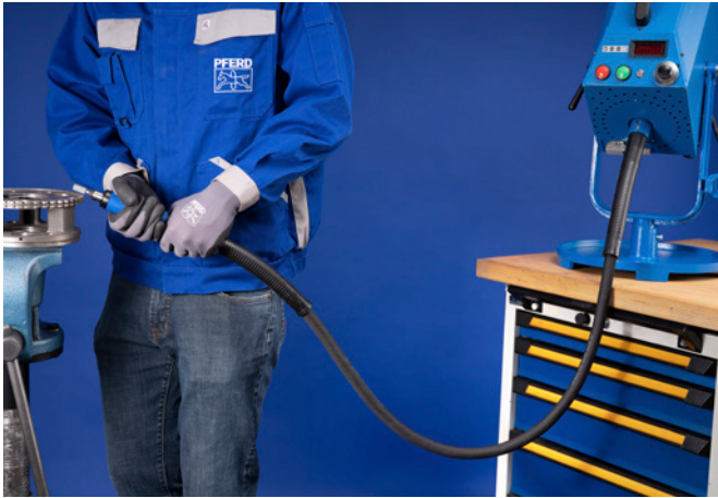
Flexible shaft drive set up correctly: flexible shaft curves gently without any bends.
